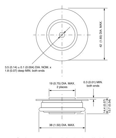
Quote between upper and lower pole pieces has to be considered after application of mounting force (see Thermal and Mechanical Specifications)
